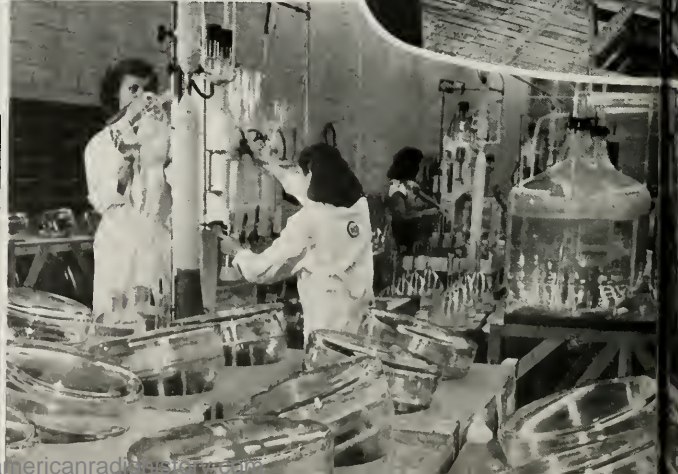
BELOW: OPERATORS PREPARE THE FLUORESCENT SOLUTION WHICH IS PLACED IN KINESCOPES TO FORM THE PICTURE SCREEN.
