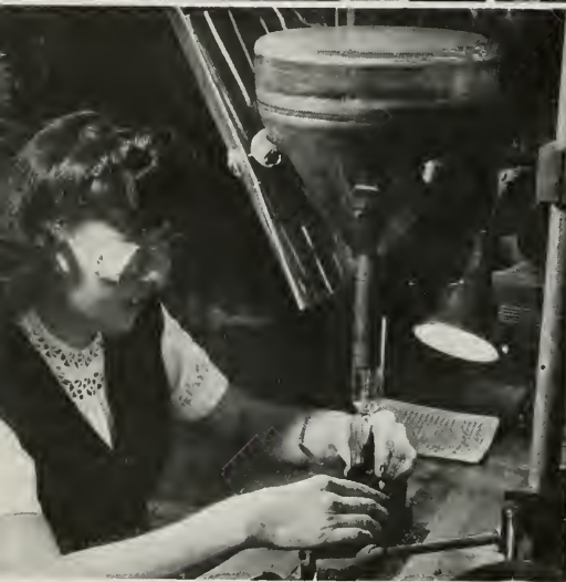
BELOW: NON-REFLECTING CARBON COATING IS APPLIED TO INTERIOR OF TUBE BY LONG-HANDED BRUSH TO KEEP STRAY ELECTRONS FROM THE PICTURE SCREEN.
