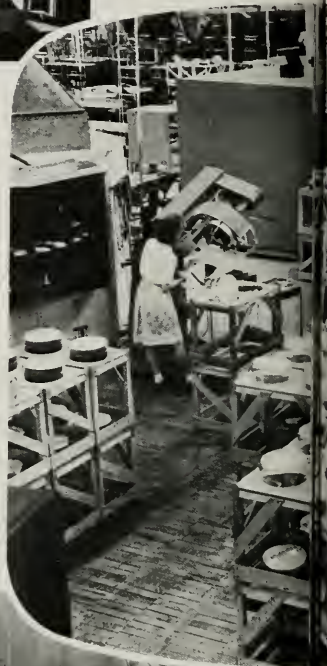
MAKING FINAL TESTS ON 10-INCH KINESCOPES USING A SPECIAL CHART AS A REFERENCE STANDARD.
